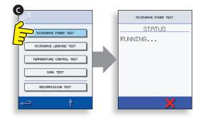
The Temperature Rise should be: e3EE & e3XE 10°C (50°F)  $\pm$ 5% e3XX 14.3°C (58°F)  $\pm$ 5%
