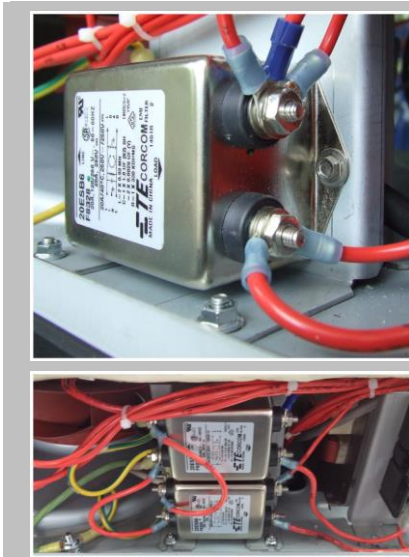
Top: one EMC filter unit (1000W e2s variant) Bottom: two EMC filter units (2000W e2s variant)
