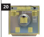
Test the areas marked in yellow above. Level must be 5mW/cm2 or lower. Record.
