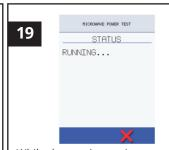
While the test is running hold the test probe at right angles to the oven and hold about 50mm away from the surface.
