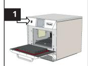
Check the oven for obvious signs of damage and cleanliness. Switch the oven on and off, allow to cool down
