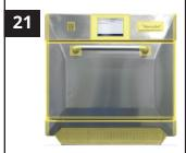
Test the areas marked in yellow above. Level must be 5mW/cm2 or lower. Record.
