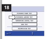
Exit out of visual view, place bowl with 275 ml of cold water in cavity and select Microwave Leakage test.
