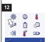
Press the spanner/tool symbol and enter the password SERVICE to access the service screen.
