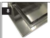
Check the door seal and ensure it is intact, not hanging loose or any sections broken away. Report defects and advise on replacement as required PSA3113.
