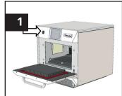
Check the oven for obvious signs of damage and cleanliness. Switch the oven on and off, allow to cool down
