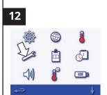
Press the spanner/tool symbol and enter the password SERVICE to access the service screen.
