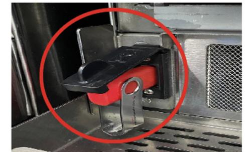
7. Insert the programmed USB into the data port. This is found behind the front filter door, left hand side.
