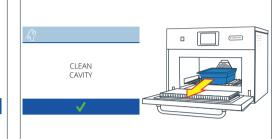
4. Once the cooling process is complete you will see a 'clean cavity' screen. Remove the pan of water. The oven is now ready for cleaning.
