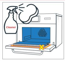
Spray Merrychef approved cleaner onto a sponge and wipe onto the sides of the inside of the oven, the back, the base, the roof and the oven door.
