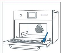
**3.** Use a dry clean brush to remove any food particles from between the cavity floor and the inside of the front door.
