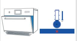
**3.** Leave the door open slightly. Wait for temperature to reduce to 50°C or 122°F. This takes approximately 20 mins.
