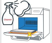
4. Spray Merrychef approved cleaner onto a sponge and wipe onto the sides of the inside of the oven, the back, the base, the roof and the oven door.
