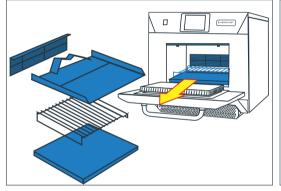
**1.** Remove the oven rack, base plate and the grease filter (pull the handle downwards and lift out). Remove the roof plate (undo the fasteners, it will drop down slightly and then pull it out).
