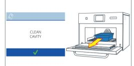
**4.** Once the cooling process is complete you will see a 'clean cavity' screen. Remove the pan of water. The oven is now ready for cleaning.
