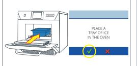
2. Place a pan of ice into the oven to speed up the cool down process. Press the green tick.
