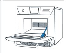
**3.** Use a dry clean brush to remove any food particles from between the cavity floor and the inside of the front door.
