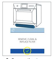
**9.** Remove the air filter and wipe it clean or wash in soapy water. Dry and replace and then press the green tick to continue.
