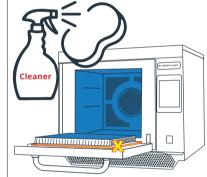
4. Spray Merrychef approved cleaner onto a sponge and wipe onto the sides of the inside of the oven, the back, the base, the roof and the oven door.
