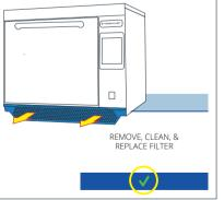
9. Remove the air filter and wipe it clean or wash in soapy water. Dry and replace and then press the green tick to continue.
