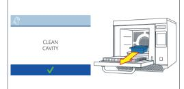
**4.** Once the cooling process is complete you will see a 'clean cavity' screen. Remove the pan of water. The oven is now ready for cleaning.
